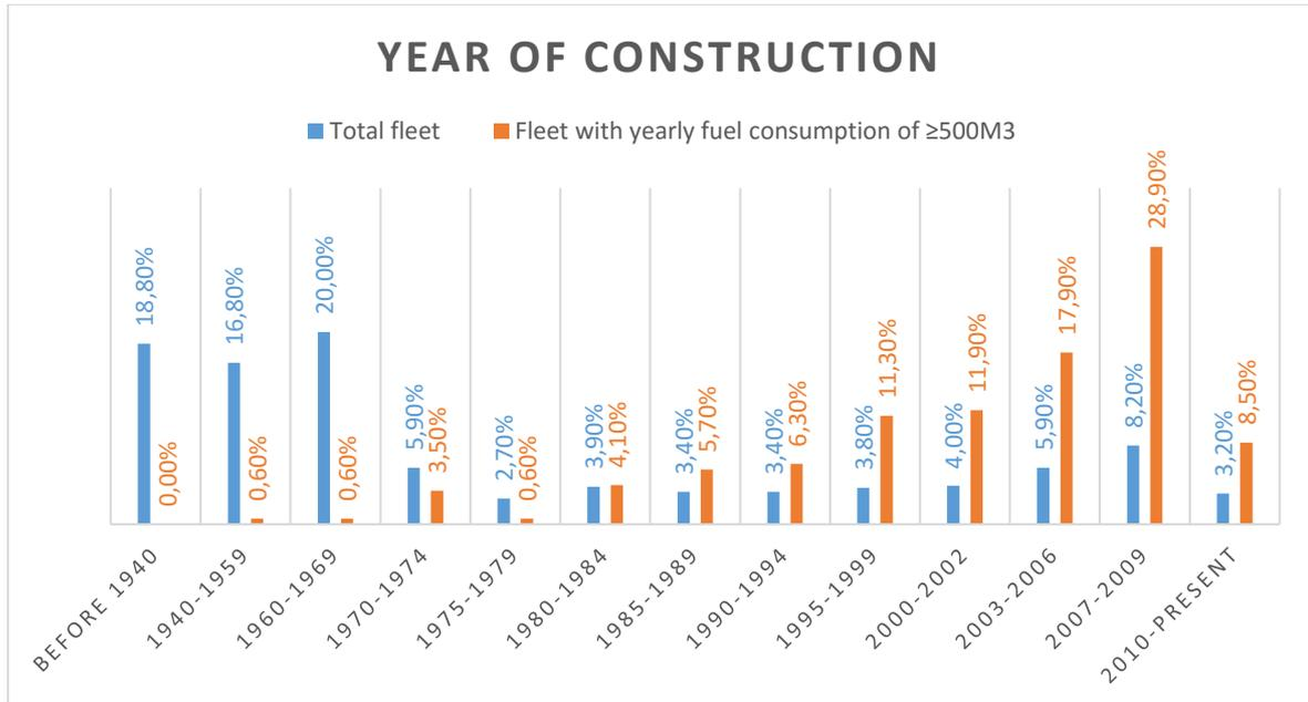
It can be seen from the figure that the fleet with a yearly fuel consumption of  $\geq 500\text{m}^3$  is relatively new. Most of these vessels were built after 2000 and a majority even in 2003 and later, which was the introduction year of CCNR Stage-1 emission norms for vessel engines. Thus, approximately 50% of the fleet with a yearly consumption of  $\geq 500\text{m}^3$  was built in or after 2004, whereas approximately 50% of the total fleet was built in or after 1965.
